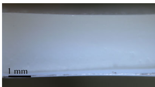
Fig. 13 Fracture surface of PA6 showing smoother morphology
